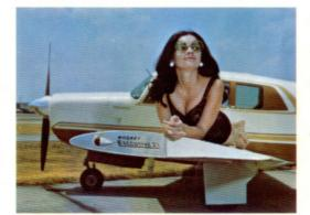
LAMINAR FLOW WING . . . This is a low-drag, high performance wing. All metal, wrap-around wing skins are flush-riveted and control surfaces are gap-sealed to minimize drag. The Mooney wing affords maximum strength and performance.
